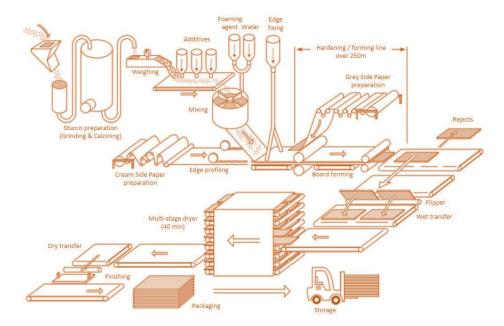
Plasterboards are manufactured using state-of-the-art production equipment and following rigorous quality assurance standards, complying with UNI EN ISO 9001:2015, as well environmental management standard complying with UNI EN ISO 14001:2015 (certified by ABICert s.a.s. with certificates reference QBC663 and ABC110 respectively). The industrial site applies also strict rules to assure health and safety for all employers and all activities in compliance with the Occupational health and safety
