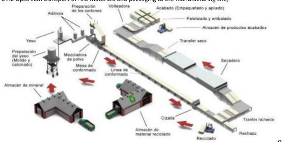
Manufacture of plasterboard (see diagram below) and production of packaging.
